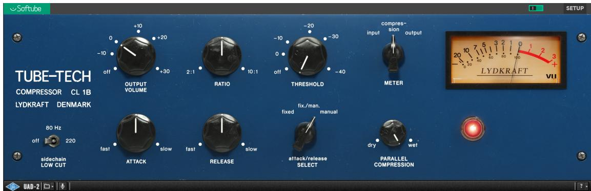
**Gain** The **Gain** control is used to “make up” for the gain loss, which takes place when the unit is compressing. It is placed after the gain reduction circuit and therefore has no influence on the threshold setting. The **Gain** control is continuously variable from off to +30 dB.
