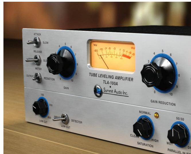
amount of saturation from the tube output stage in the compressor. Without it, you would have to use the Gain control to set the desired amount of distortion and compensate for that loss or increase in volume with a separate volume control. The Saturation does all that. In one knob.
