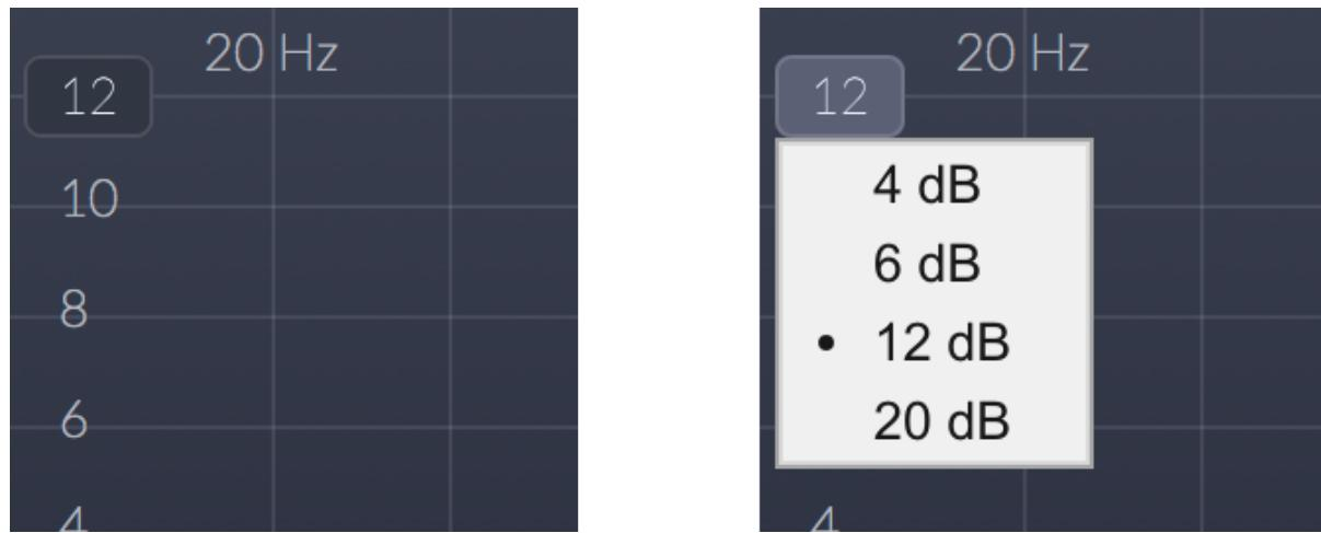
Toggle the graph dB scale between -/+4 dB, -/+6 dB, -/+12 dB and -/+20 dB scales.
