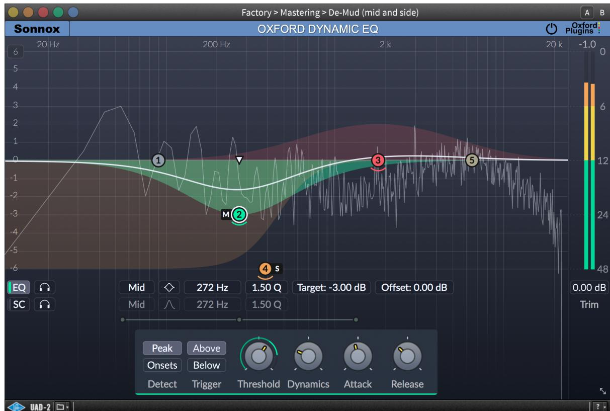
Equalisation is the audio engineer's most widely used processing tool. However, the equalisation applied is usually static – it remains the same over time.
