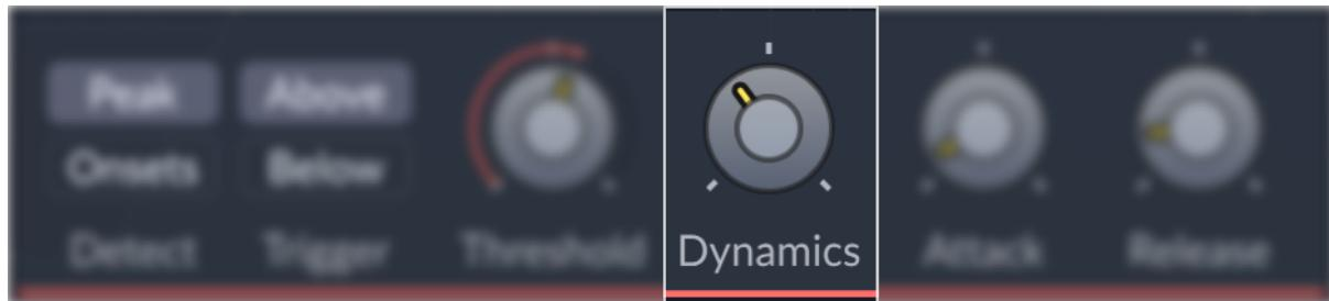
Set how reactive the band's gain is. This is similar to a compressor's ratio control.
