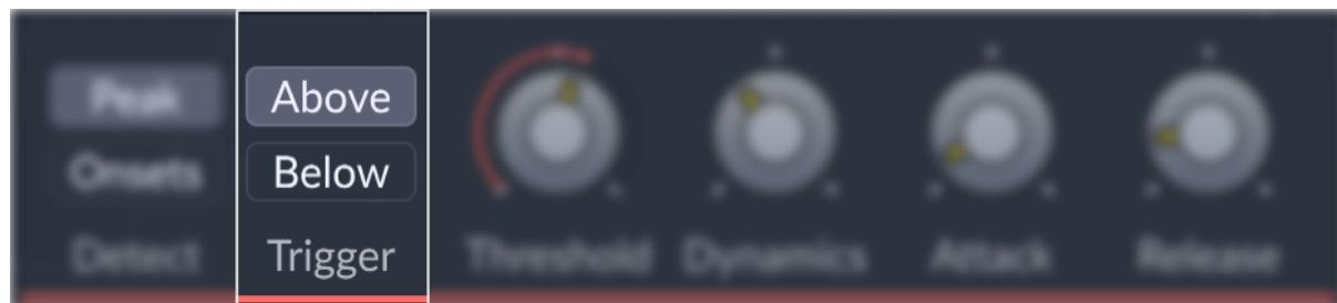
In Above mode, gain changes dynamically when the signal is above the Threshold. Use Above mode for downwards compression and upwards expansion.
