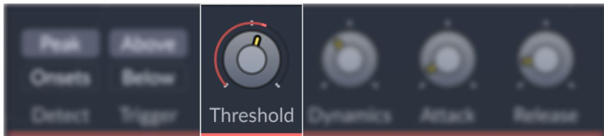
Set the level at which the dynamics processing becomes active (depending on the Trigger setting).
