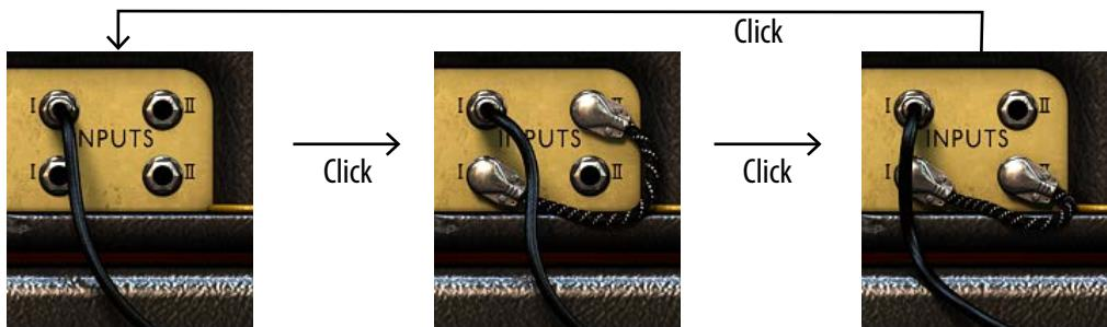
*Black cable (guitar) in Input I High input, no patching between channels. Click on the input to select the first patch configuration, or another input to select a different input.*
