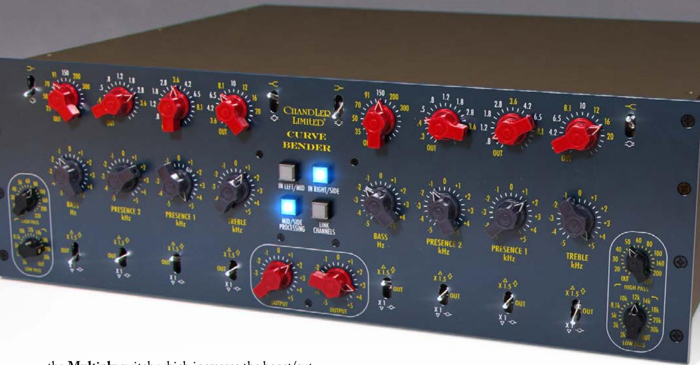
the **Multiply** switch which increases the boost/cut ability from 5 to 15 dB, as well as sharpening the Q. He furthermore added high and low pass filters, and bell/shelf selections on the high and low bands.
