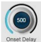
Sets the amount of time in milliseconds between the beginning of a note and the onset of vibrato. The range is from 0 to 1500ms (1.5 seconds).
