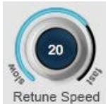
Retune Speed controls how rapidly the pitch correction is applied to the incoming sound. The units are milliseconds. A zero setting will cause immediate changes from one pitch to another, and will completely suppress any vibration.
