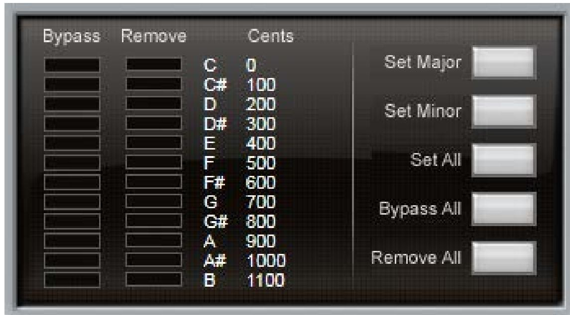
The Edit Scale Display is used to create custom scales or to modify any of the preset scales selected in the Scale menu
