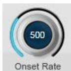
Sets the amount of time in milliseconds between the end of the onset of vibrato and the point at which the vibrato reaches the full values set in the Pitch, Amplitude and Formant Amount settings. The range is from 0 to 1500ms (1.5 seconds).
