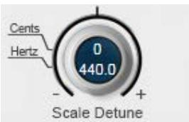
The Detune parameter allows you to change the pitch standard of Auto-Tune Realtime from the default A = 440Hz. This is useful when working with an instrument or track that uses a different reference frequency. Values are specified in both cents and Hertz. The range of adjustment is -100 cents to +100 cents.
