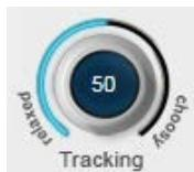
In order to accurately identify the pitch of the input, Auto-Tune Realtime requires a periodically repeating waveform, characteristic of a solo voice or solo instrument. The Tracking control determines how much variation is allowed in the waveform for Auto-Tune Realtime to still consider it periodic.
