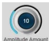
Sets the amount that the loudness changes. For the most realistic vibrato, the amount of amplitude change should be substantially less than pitch change. The range is from 0 (no change) to 30 (maximum change).
