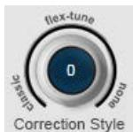
The Correction Style control lets you select either the classic Auto-Tune style pitch correction or our new Flex-Tune technology, which provides pitch correction while preserving a singer's expressive vocal gestures.
