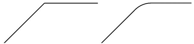
The Attack Time Control is used to set how quickly the compressor applies the gain reduction, at its minimum (70uS) the gain reduction is applied extremely quickly with a more audible effect, at its maximum (50mS) the change in gain is more gradually applied.
