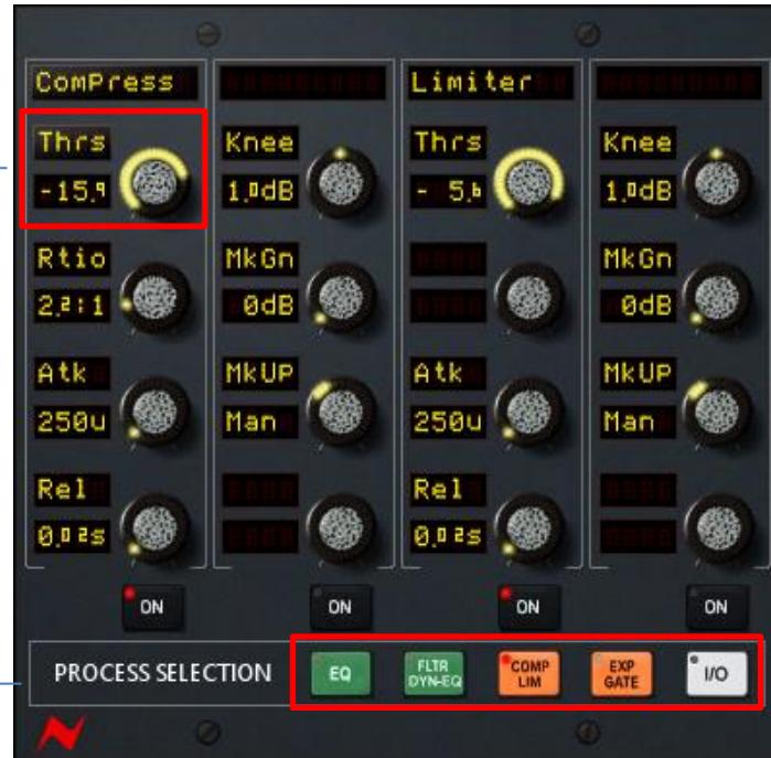
Processes are assigned in horizontal 'Strips' comprising Process Name, 4 Controls and an 'On' button.
