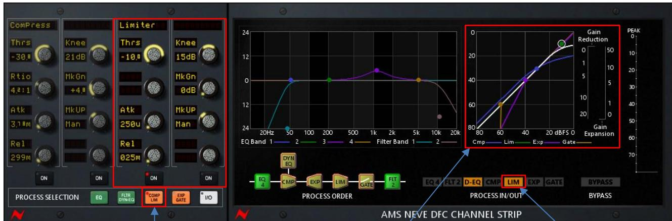
To access the Limiter controls, select the Comp/ Lim Process Selection button, the 3<sup>rd</sup> and 4<sup>th</sup> strips of the Chan-Quad are then assigned to the Limiter Controls. The 3<sup>rd</sup> 'On' button is assigned to the Compressor In/ Out control.
