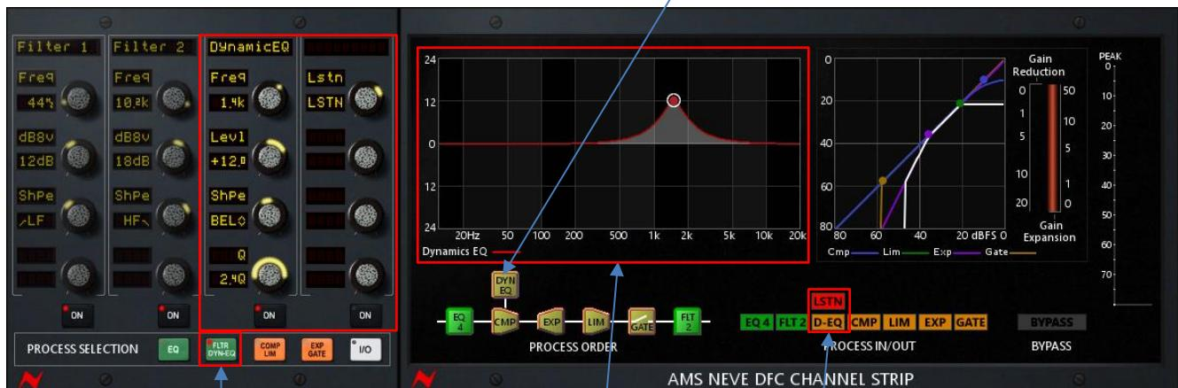
To access the Dynamics EQ controls, select the Filter/ Dyn-EQ Process Selection button, the 3<sup>rd</sup> and 4<sup>th</sup> strips of the Chan-Quad are then assigned to the Dynamics EQ Controls. The 3<sup>rd</sup> 'On' button is assigned to the Dynamics EQ In/ Out control.
