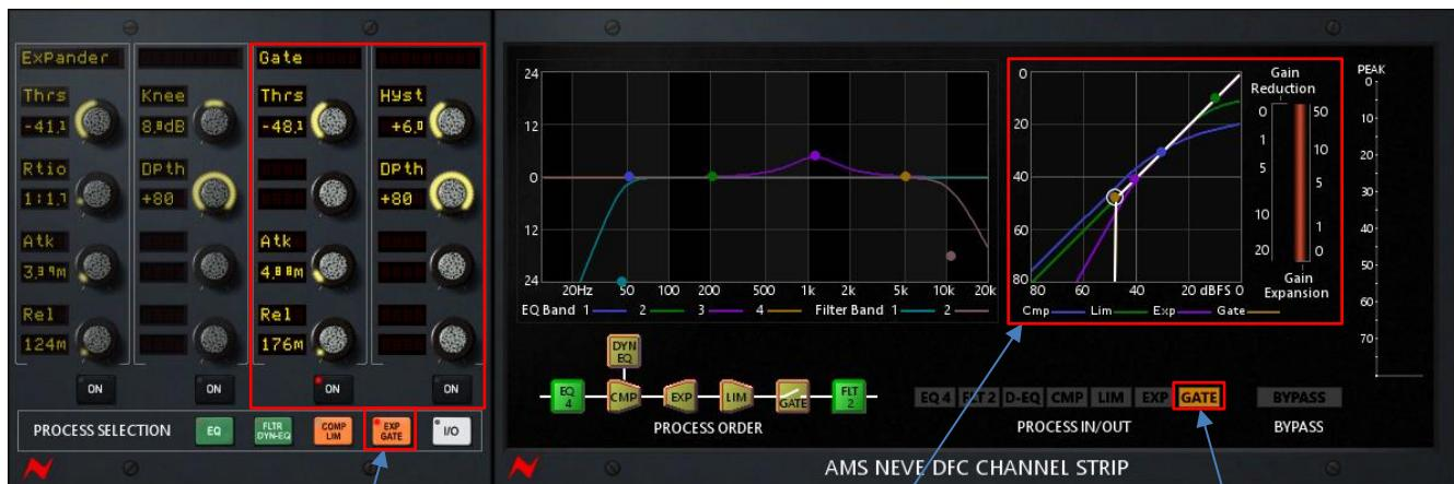
To access the Gate controls, select the Exp/ Gate Process Selection button, the 3<sup>rd</sup> and 4<sup>th</sup> strips of the Chan-Quad are then assigned to the Gate Controls. The 3<sup>rd</sup> 'On' button is assigned to the Gate In/ Out control.
