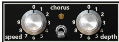
*When the chorus is on, pitch controls are locked out, as the pitch is being used by the chorus feature.*
