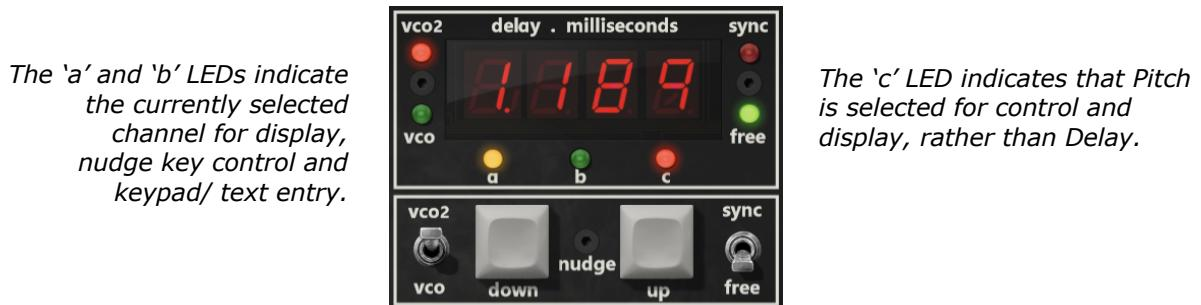
Keyboard entry of Delay and Pitch values can be achieved by clicking on the 7-segment display area and entering the required value on the computer keyboard, followed by the enter key.
