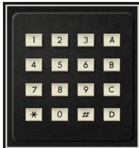
*Pitch values can be entered with the keypad as a ratio of the original pitch within the range of 0.5 and 2.0. Use the '\*' button as a decimal point and '#' as 'execute'.*
