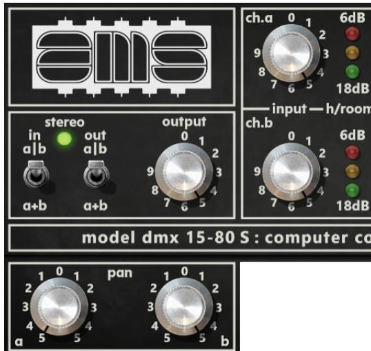
*In mono instances, the configuration switches are forced to 'a+b'. If only one channel is needed, the unused channel input gain may be set to zero.*
