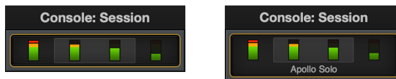
Meter Bridge with Show Device Names OFF (left) and ON (right)
