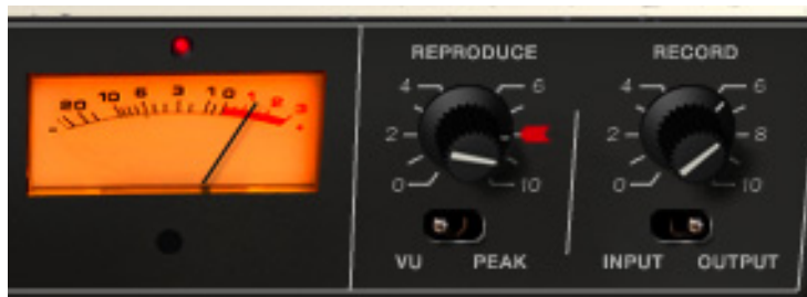
Figure 46. One side of the Ampex ATR-102 “penthouse” showing meter and I/O controls
