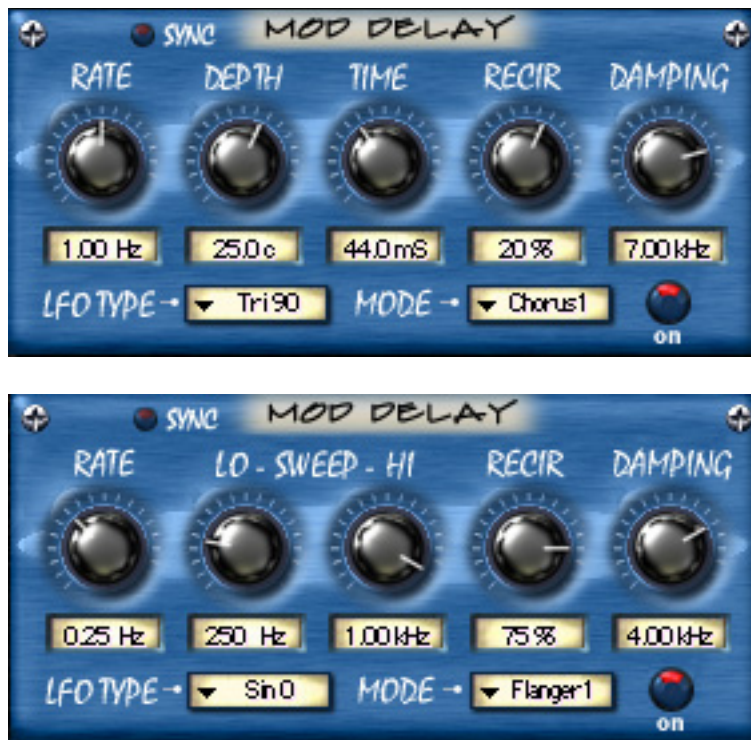
Figure 137. The Mod Delay module The label and function of the second two knobs depend upon the Mode menu selection.
