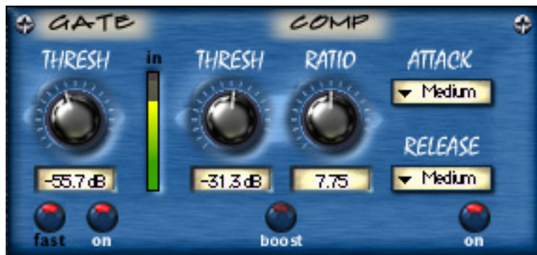
Figure 130. The Gate/Comp module
