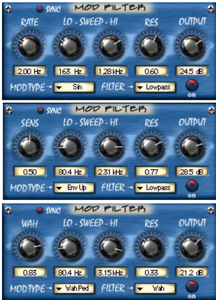
Figure 134. The Mod Filter plug-in window The label and function of the first knob depends upon the Mod Type menu selection.
