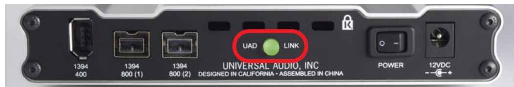
Figure 31. UAD-2 LED on Satellite rear panel
