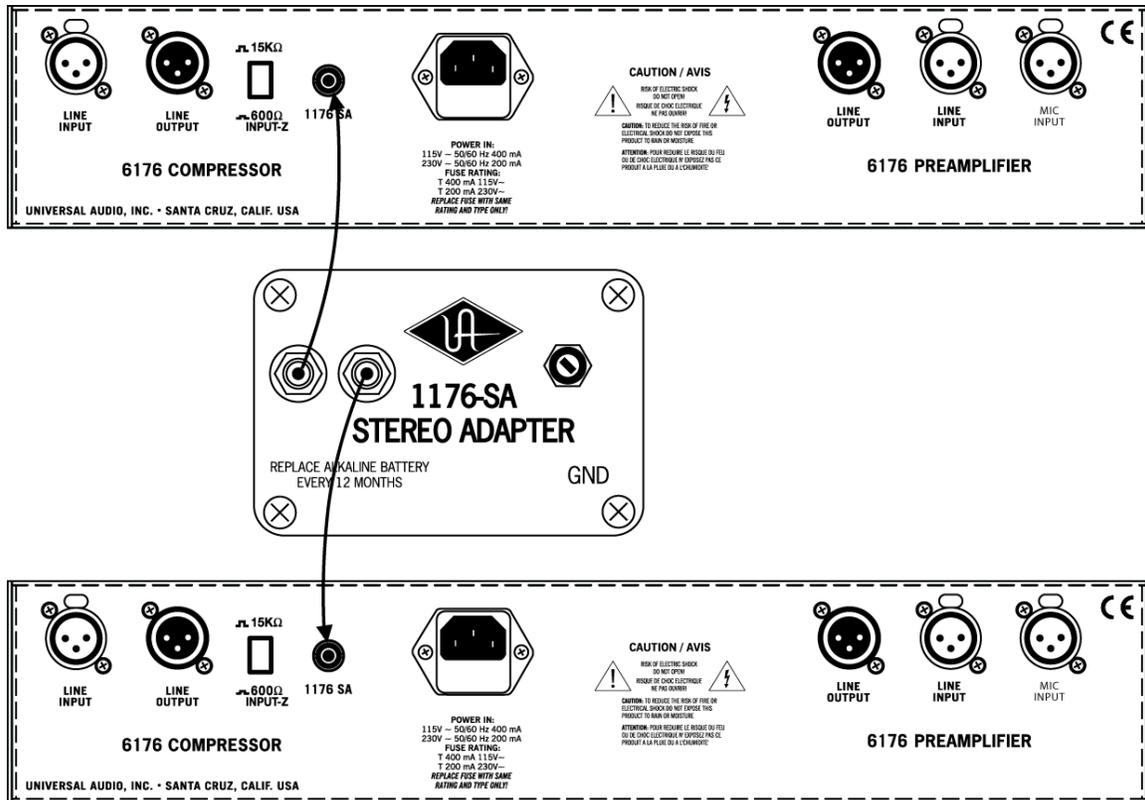
**Note:** When used in stereo operation, the Attack and Release controls on the two 6176s will interact so that changing the Attack or Release times on either device changes that of both devices. Note that when connected in a stereo configuration, the fastest attack time is doubled (that is, it becomes 40 microseconds instead of 20 microseconds).
