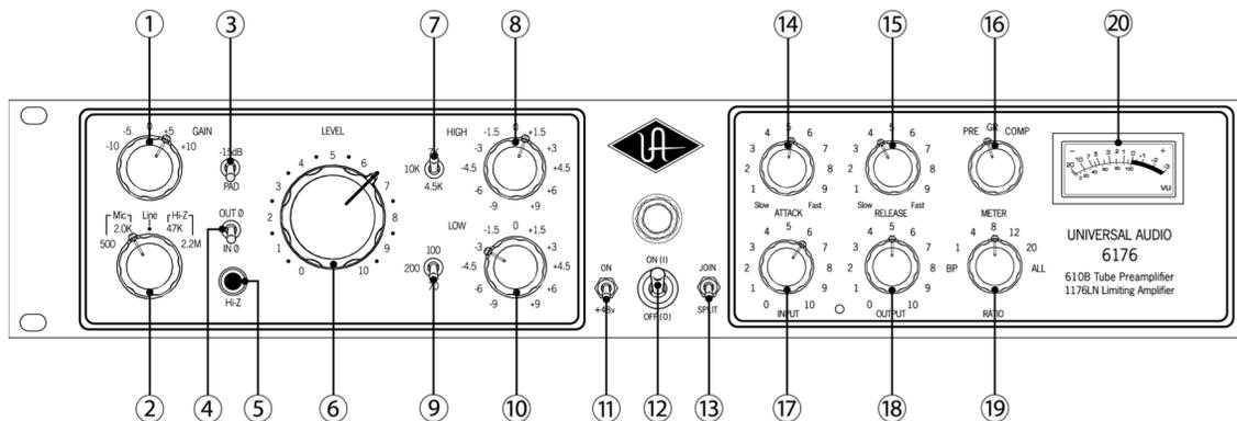
**NOTE:** The left side of the 6176 front panel contains all preamp controls, while the right side contains all limiter / compressor controls. All controls (except the Level, Attack, Release, Input, and Output knobs) are stepped, allowing settings to be easily reproduced.
