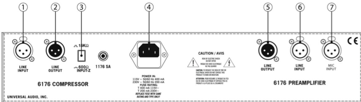
**(1) Limiter / Compressor LINE INPUT** - Connect a line-level input signal (coming from a device such as a mixer, DAW, tape machine, or signal processor) to the limiter/compressor section via this balanced XLR connector. Pin 2 is wired positive (hot).
