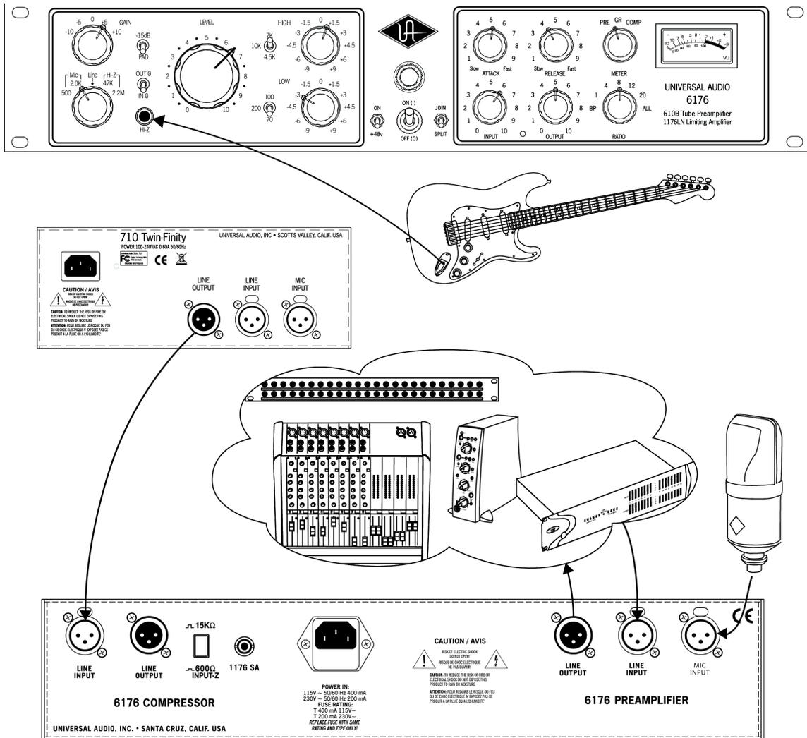
**i** When operating in JOIN mode, the rear panel Preamp LINE OUT and the Limiter/Compressor LINE IN jacks are automatically disconnected.
